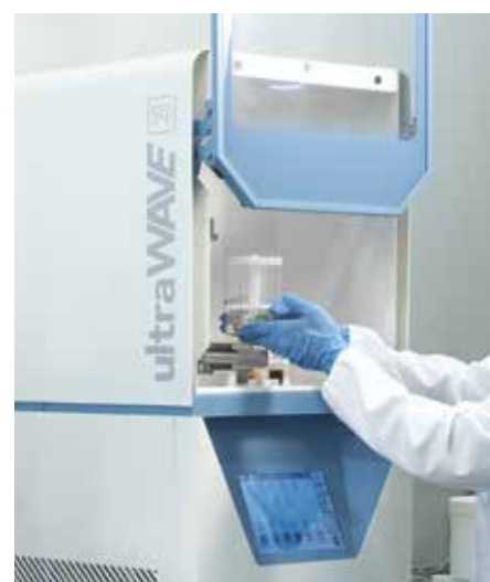
Vessels are ready for the digestion process
